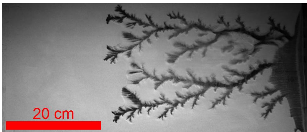
Fig. 1 : Top-down view of aerofractures in the Hele-Shaw cell
